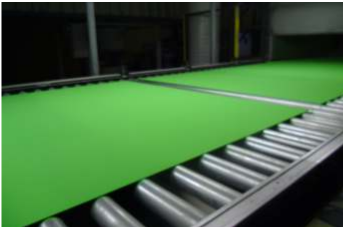
Continuous sheet coating line
